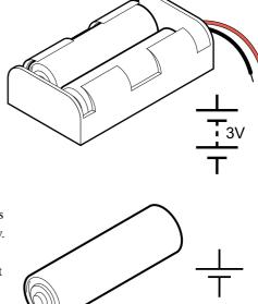
AA cells will last much longer than a 9V PP3 battery, as it contains a larger total amount of chemical energy as it is physically larger. Therefore items that require more power to work (e.g. a CD walkman which contains a motor and laser to read the CD's) will always use AA cells rather than PP3 batteries.
