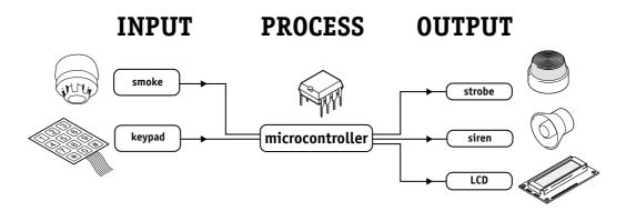
The smoke sensor and keypad provide information to the microcontroller, and so these are known as 'inputs'. The microcontroller then 'decides' how to behave and may then operate the outputs e.g. make the siren and strobe switch on or display a message on the Liquid Crystal Display (LCD).
