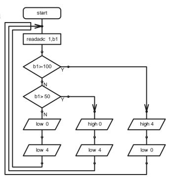
The 'readadc' command is used to read the analogue value (a number between 0 and 255) into variable b1. Once the number is in variable b1 it can be tested to see if it is greater than 100 or greater than 50. If it is greater than 100 output 4 is switched on, if it is between 50 and 100 output 0 is switched on, and if it is less than 50 both outputs are switched off.
